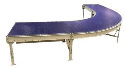
Systec's Stable Stack Bundle Conveyor (SSBC) is a material handling solution for applications in which a smooth surface is required. The SSBC Curve has advantages over standard bundle conveyor curves because it eliminates the gap between rollers and product maintains a 90 degree orientation.
